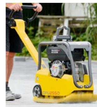
**Top-Speed-Version:** for high surface performance in laying paving stone.
