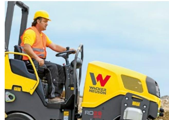
**Optimum view** due to the laterally adjustable seat.
